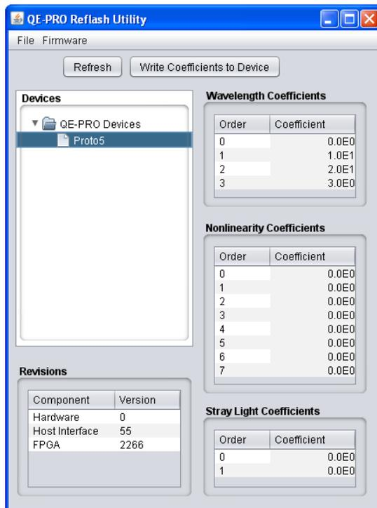
6. Double-click on each of the calibration coefficients displayed in the **Wavelength Coefficients** pane of the USB Programmer screen and enter the new values acquired in Step 5 of the [\*Calibrating the Wavelength of the Spectrometer\*](#) section in this appendix.
