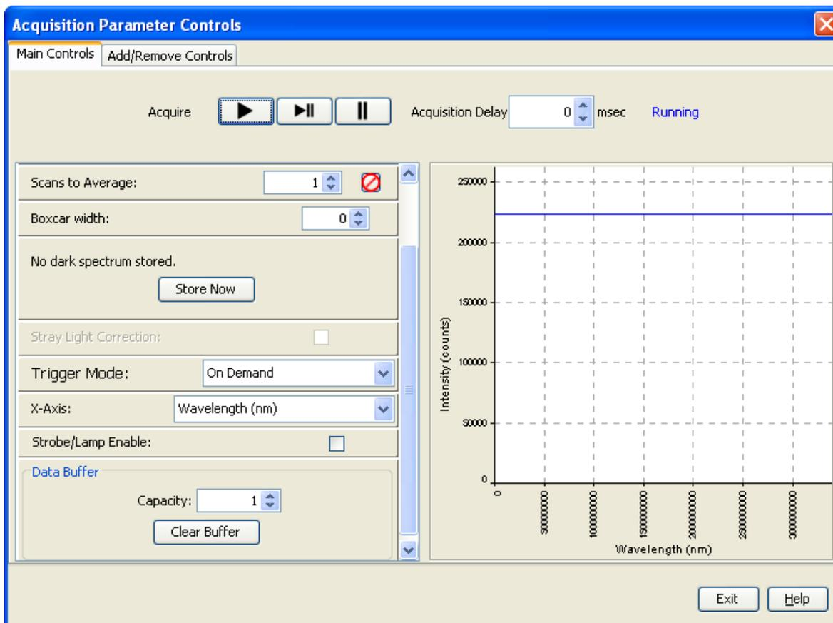
3. Select the data buffering capacity (the total number of scans the device can store at once).
